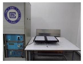
7.5. Photo of electrostatic discharge Immunity measurement (E.S.D.)
