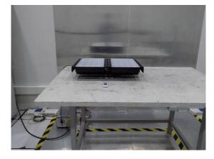
7.2. Photo of radiated emission measurement (R.E. Magnetic field)
